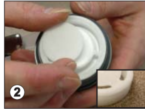
Locate recessed area on filter cassette top and remove impaction substrate. If chemical analysis of larger particles is desired, place in appropriate container for shipping to a laboratory for analysis. See Accessories for Filter-Keeper.
