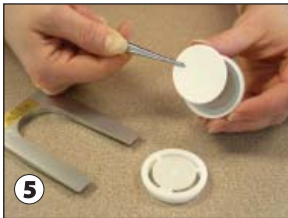
Use the forceps accessory to remove the final collection filter and place it in an appropriate container for shipping to a laboratory.
