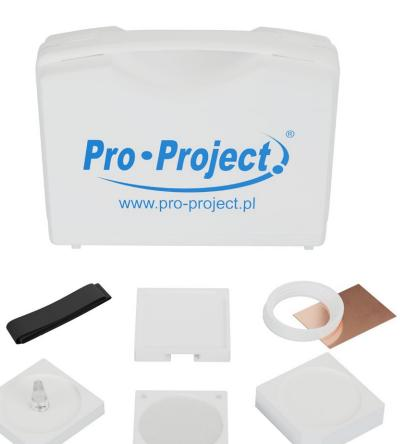
This kit is a versatile set of phantoms and software for carrying out constancy tests of intra-oral and OPG dental X-ray units. Thanks to the Pro-Control.online subscription, all tests can be quickly and effortlessly automatically analysed online.
