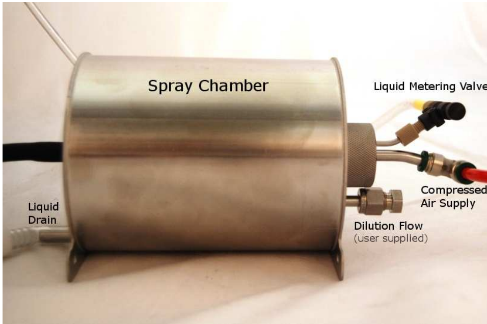
Figure 3: Photo of spray chamber showing filtered air supply input line (1/4" outside diameter tube) and liquid supply input line (1/8" outside diameter tube). Note the position of the liquid metering valve ABOVE the compressed air supply fitting.
