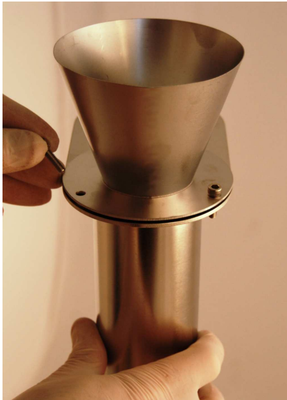
Figure 10: View of funnel attached to in-line dryer.
