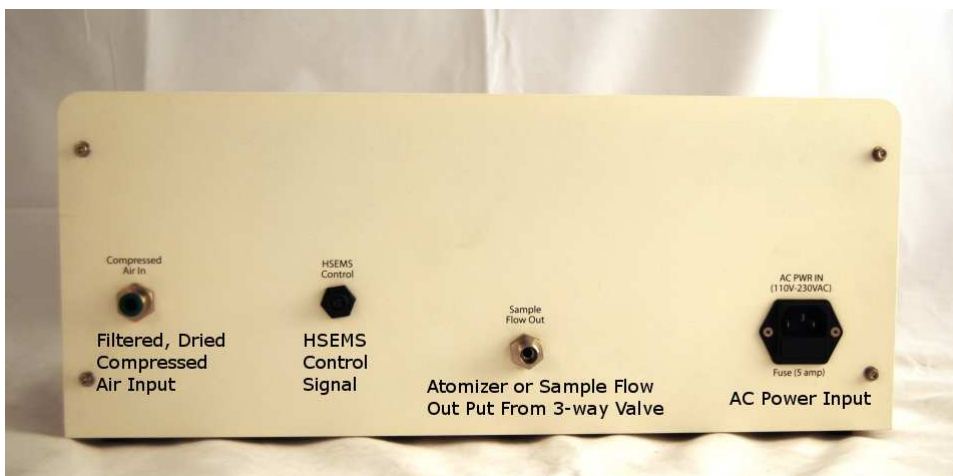
Figure 5: Rear of the Auto-atomizer chassis showing the AC power input, atomizer or user inlet outlet, HSEMS control signal input and the compressed air input to the atomizer.
