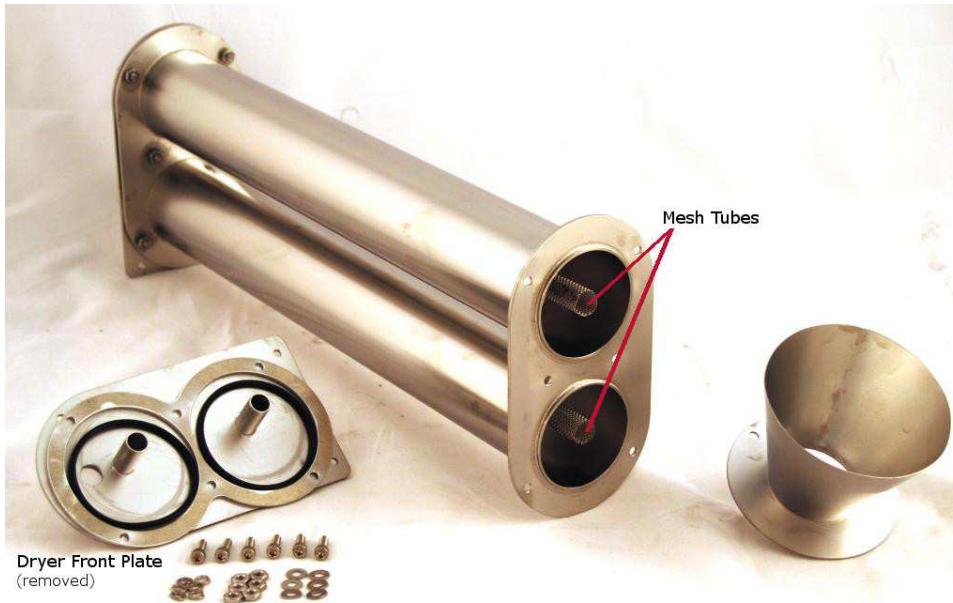
Figure 7: View of open in-line dryer.
