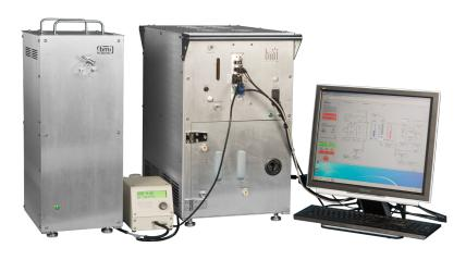
Real-time particle size and relative humidity dependent hygroscopic growth and number distribution measurement system
